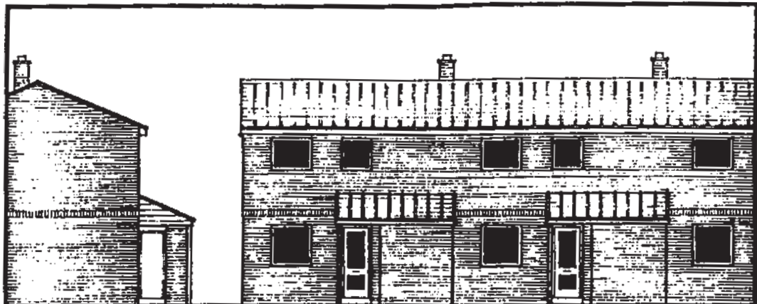
PART END PART FRONT ELEVATION CLEAN DESIGN. IMPROVED INSULATION. ATTENTION TO DETAILS TO REDUCE MAINTENANCE COSTS. HIGH PERFORMANCE WINDOWS. RATIONALISED TRAD. 1975 PLATE 9
