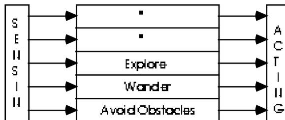
Figure 7 - Brook’s Subsumption Architecture
